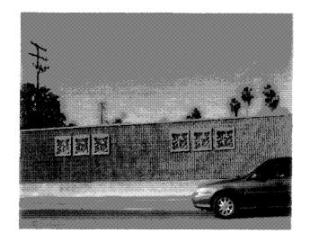
Soundwalls have minimal effect when receivers are more than 250 ft away
