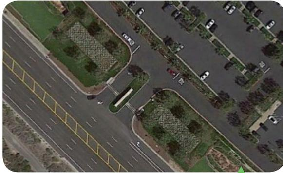
Construct a raised median at the shopping center entrance near Crystal Heights Drive to preclude illegal turns across the striped median \$\$
