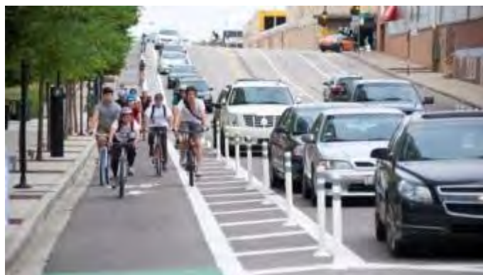
Figure 2.5: Class IV Bicycle Facility
