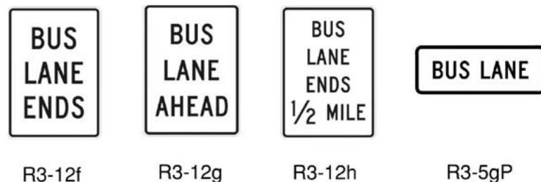
Figure 44: Bus lane alert signs-pole/signal mast arm mounted (MUTCD).
