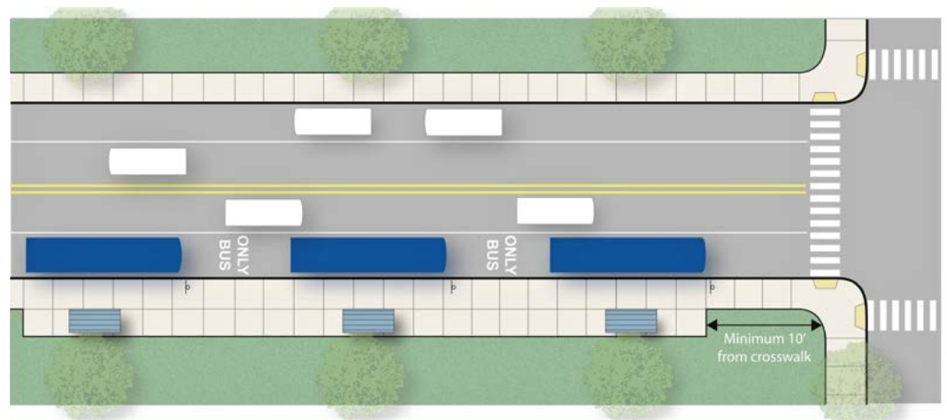
Figure 18: Conceptual configuration of a multi-route layover zone.
