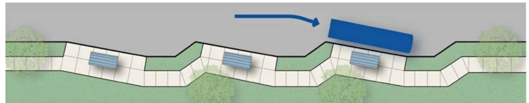
Figure 19: Conceptual example of a sawtooth arrangement of a multi-route layover zone.
