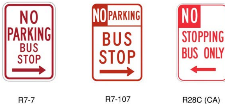
Figure 46: No parking / stopping signs to delineate bus stop zones (CA MUTCD).
