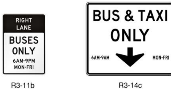
Figure 45: Part-time bus lane alert signs (CA MUTCD).
