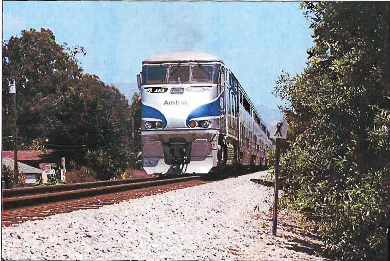
Figure 2-3: Amtrak train traveling southbound in “Push” mode (note the red lights indicating the “rear” of the train)
