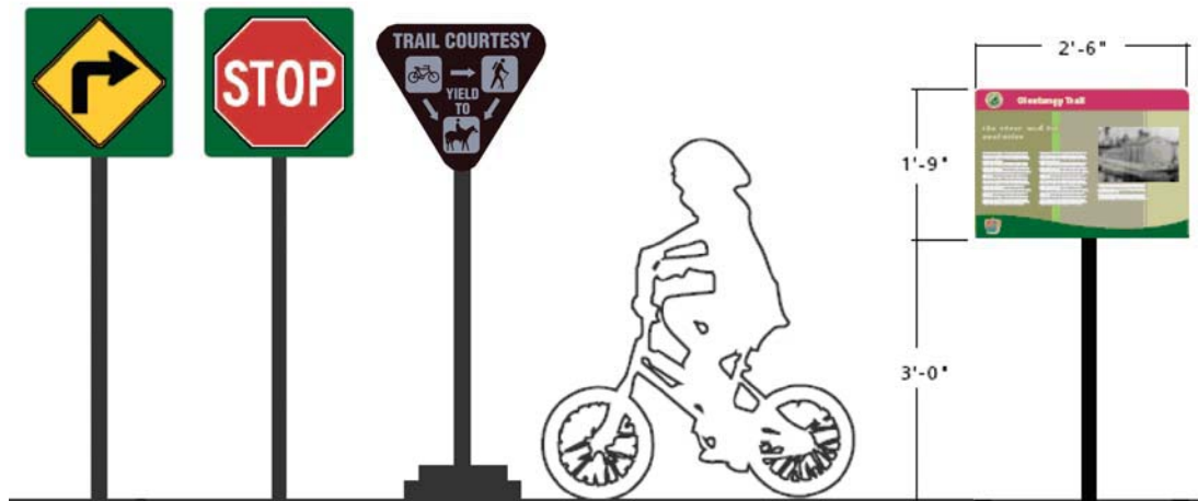
Figure 2.12: Multi-Use Path Signs
