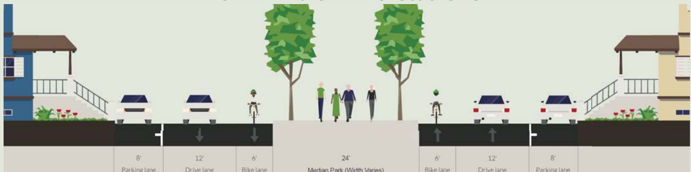
Proposed cross section of Electric Avenue left side bike lanes
