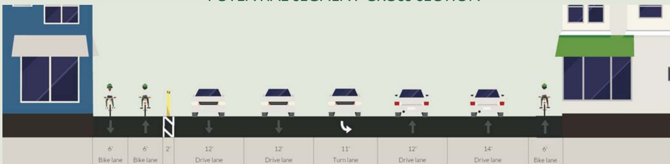
Proposed cross section for Pacific Coast Highway west of Anderson Street.
