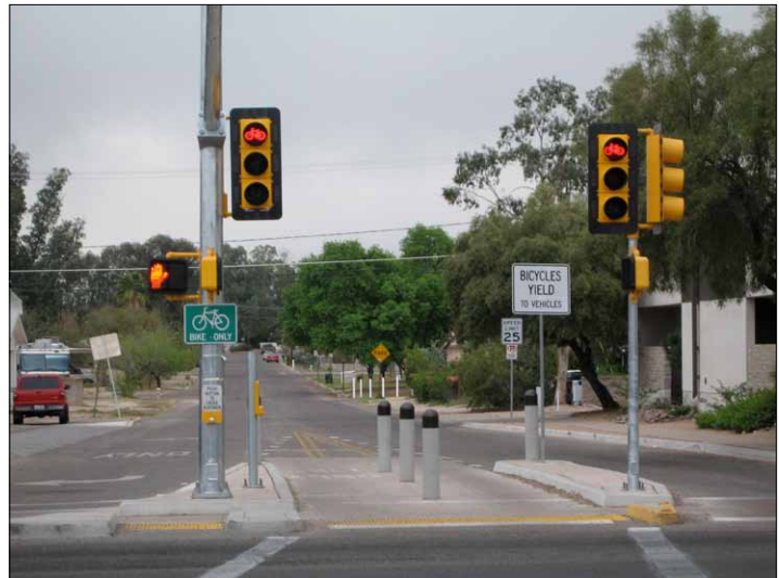
Bicycle Signals (Tucson, AZ) Photo credit: John Holloway
